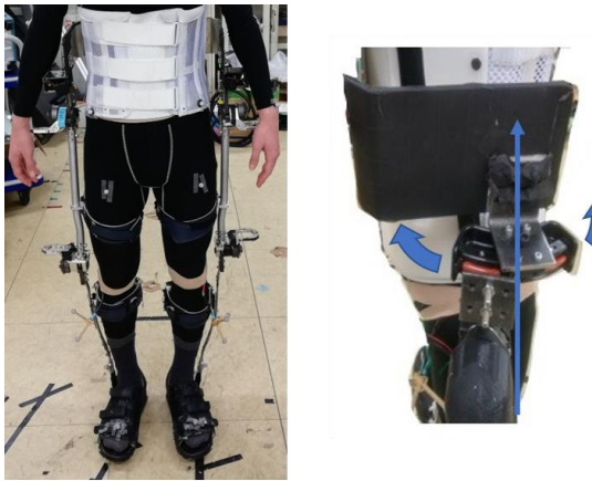
(a) Overview (b) Hip rotation joint
