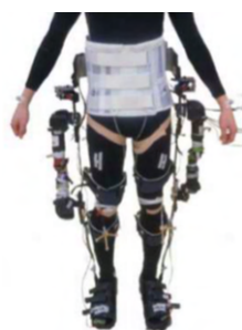
Fig.2 MALO: Motor Actuated Lower-limb Orthosis
